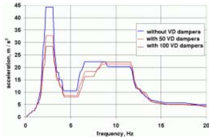
*Fig.30 The Seismic Broaden Response Spectra for the Containment Gallery of the Reactor Building (Damping 2%)*
