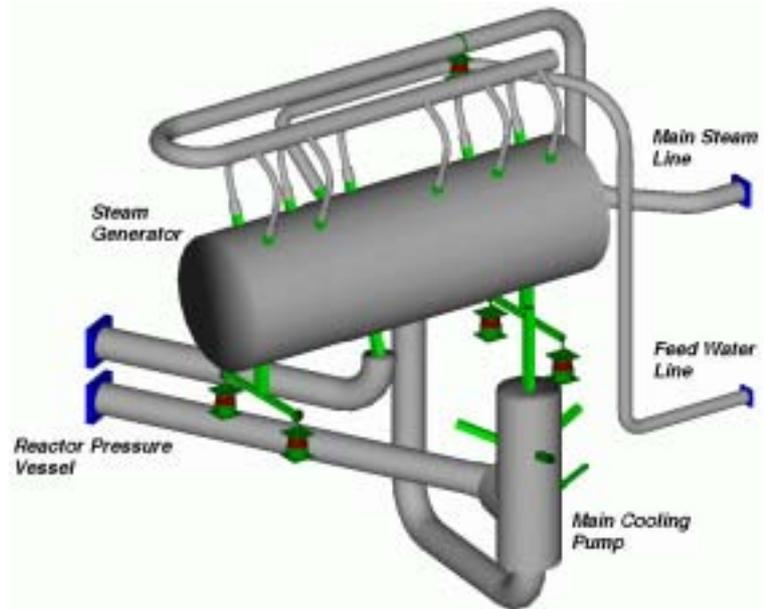
*Fig.2 VD-Dampers Installed on Primary Coolant Loop of NPP (Reactor Building)*
