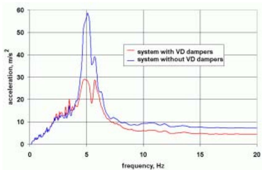
*Fig.9 Acceleration Response Spectra for “Envelope – Internal Structures” System with 90 VD Dampers and without Them (Two Oscillators)*
