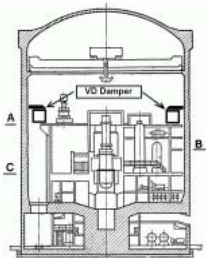
Fig.12 Vertical Section of NPP Reactor Building. The Installation of Dampers
