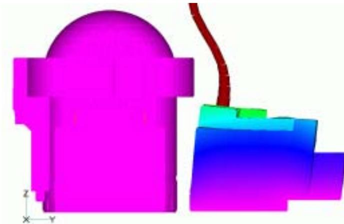
Fig. 28 General Mode Shape of the Special Building (7.66 Hz)
