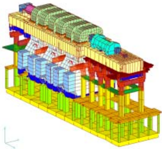
Fig. 16 Mode Shape № 1 of BVT System (1.30 Hz)
