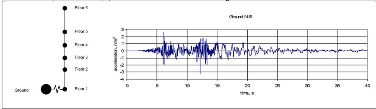
Figure 6 Stick model of the reactor building and N-S accelerogram of ground motion
