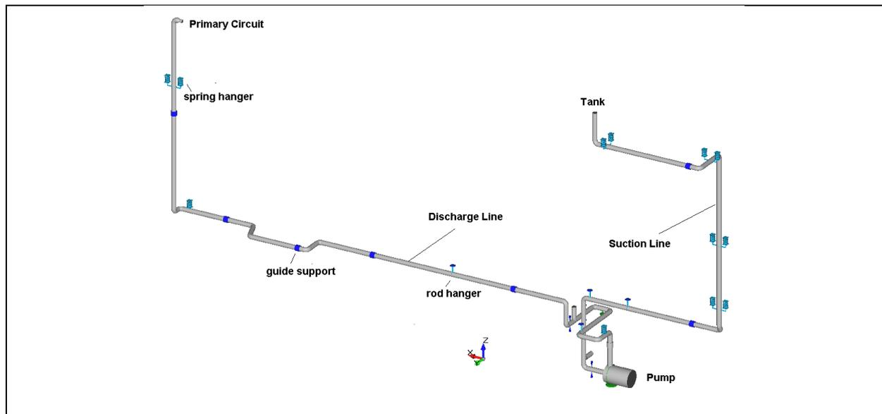
Figure 5 FE model of the pipeline
